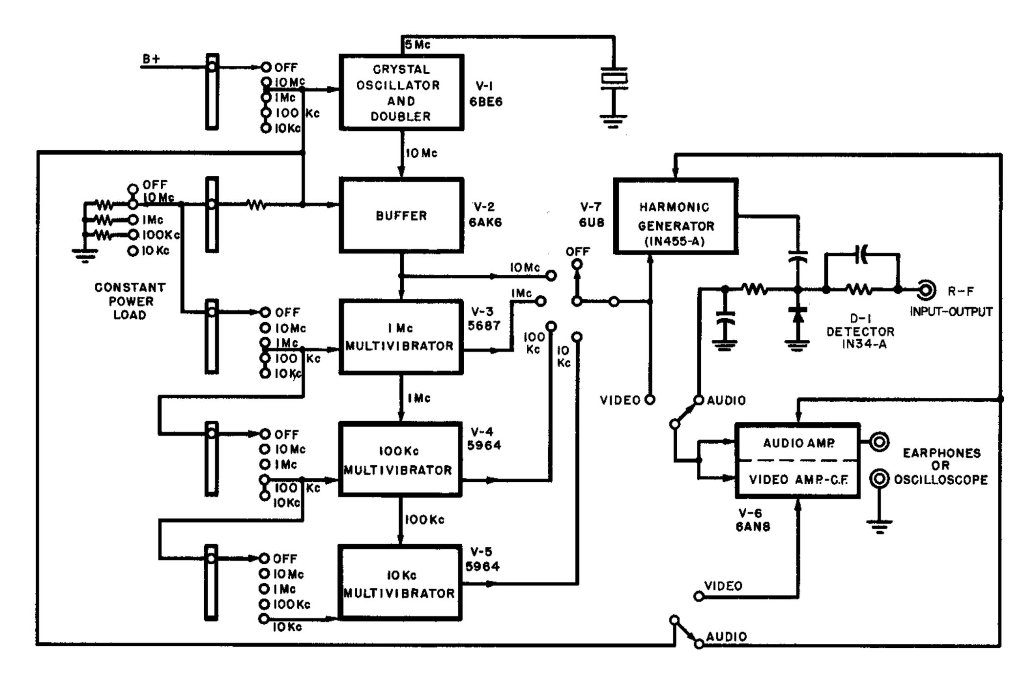
Figure 2. Block Diagram of Type 1213-C Unit Time/Frequency Calibrator.
